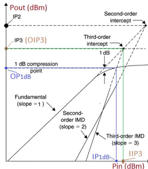
In a power sense ( $V^2$  is a power quantity), a factor of 0.10875 corresponds to  $-9.636 \text{ dB}$ , so by this approximate analysis, the 1 dB compression point occurs roughly 9.6 dB below the TOI.
