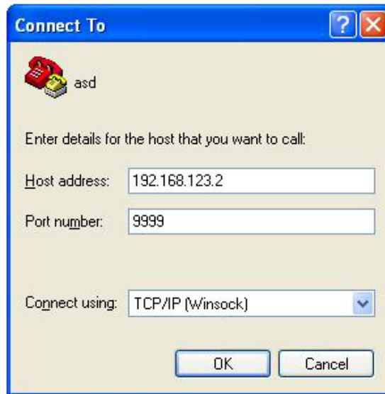
Figure 1-E Telnet® Settings in Hyper Terminal
