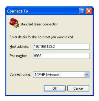
Figure 2-E: Telnet® Settings in Hyper Terminal
