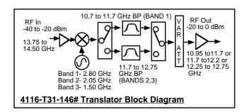
FIGURE 1 Model 4116-T31-146# Multi-Band Block Translator Block Diagram
