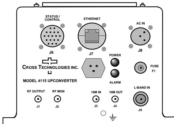
**Model 4115-41-212 Ka-Band Block Upconverter Front Panel**
