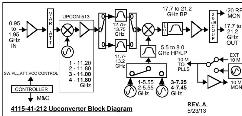
**FIGURE 1.0 Model 4115-41-212 Ka-Band Upconverter Block Diagram**
