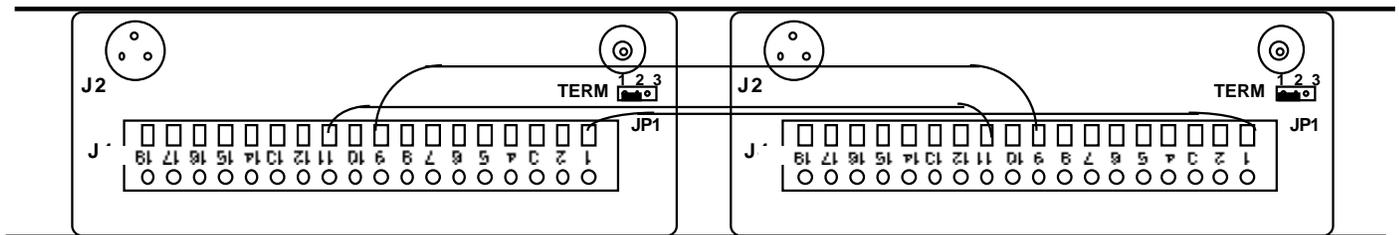
**FIGURE 2.6 Model 27XX Rear Panels Showing DC wired together for Use With One Wall Power Supply**
