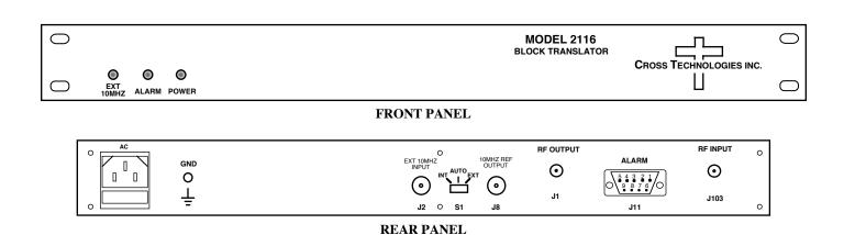
FIGURE 1.1 Front and Rear Panels
