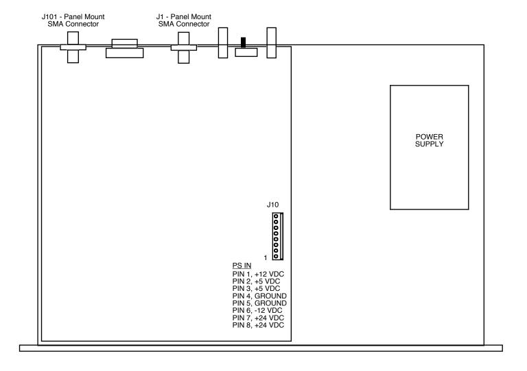
FIGURE 2.0 2116-140T120 Mechanical Assembly
