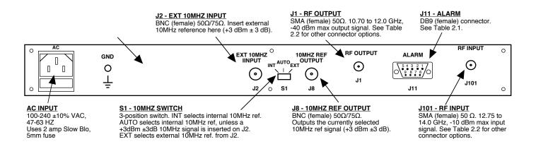
FIGURE 2.1 2116-140T120 Rear Panel I/O's
