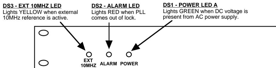
**FIGURE 2.2 2116-116 Front Panel Controls and Indicators**
