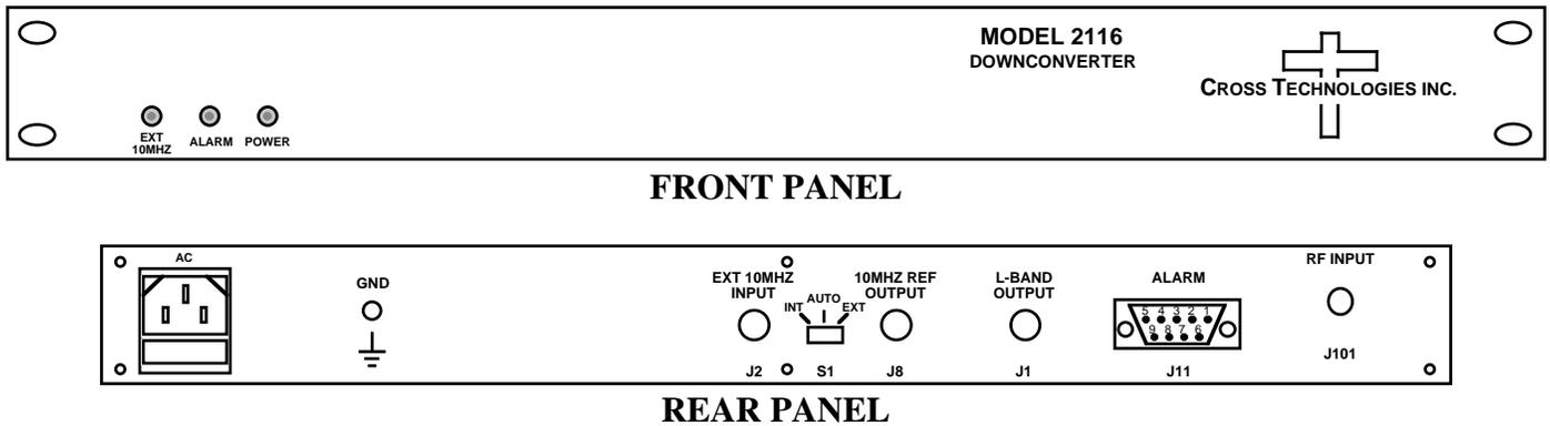
**FIGURE 1.1** Model 2116-116 Front and Rear Panels
