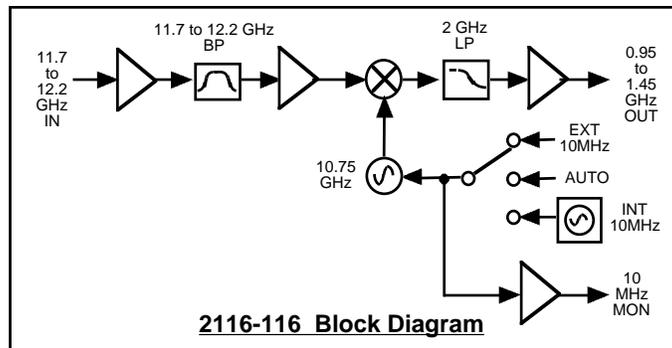
**FIGURE 1.2** Model 2116-116 Downconverter Block Diagram
