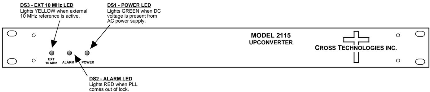
**FIGURE 2.2 Front Panel Controls and Indicators**
