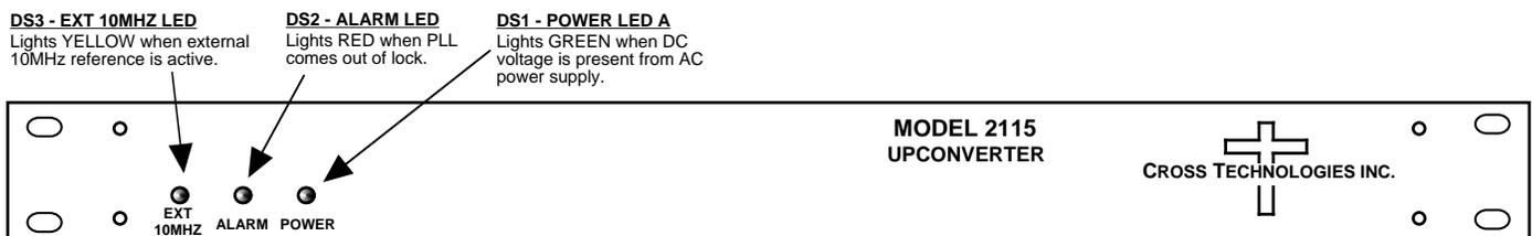
**FIGURE 2.2 2115-275-1845 Front Panel Controls and Indicators**
