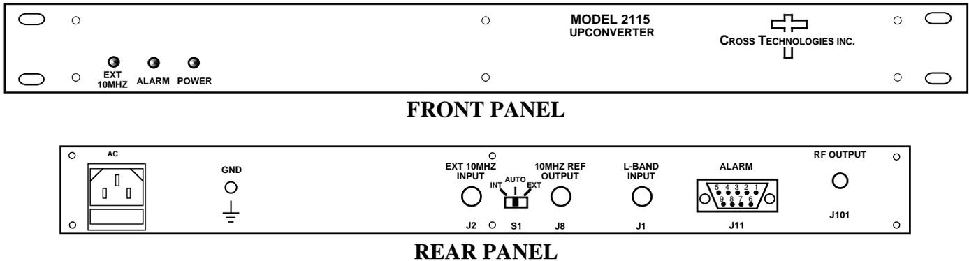
FIGURE 1.1 Model 2115-275-1845 Front and Rear Panels
