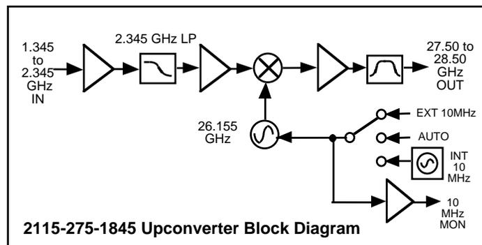
FIGURE 1.2 Model 2115-275-1845 Upconverter Block Diagram
