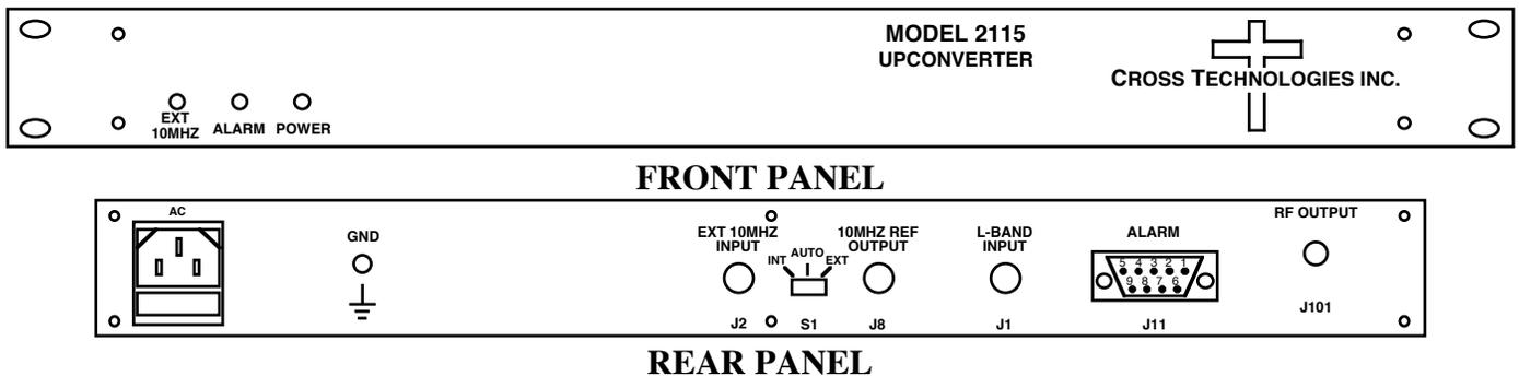
**FIGURE 1.1 Model 2115-140 Front and Rear Panels**
