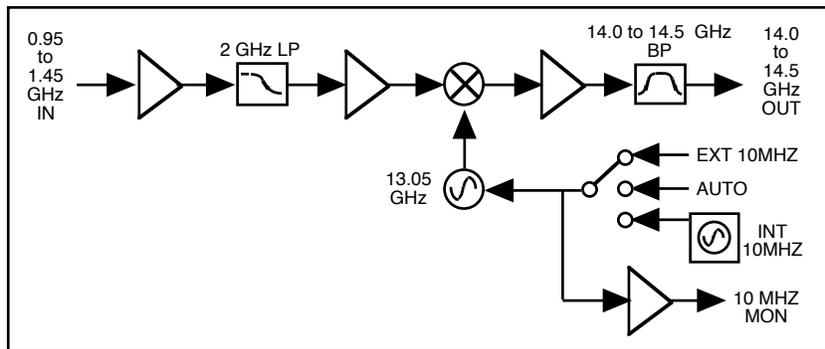
**FIGURE 1.2 Model 2115-140 Upconverter Block Diagram**
