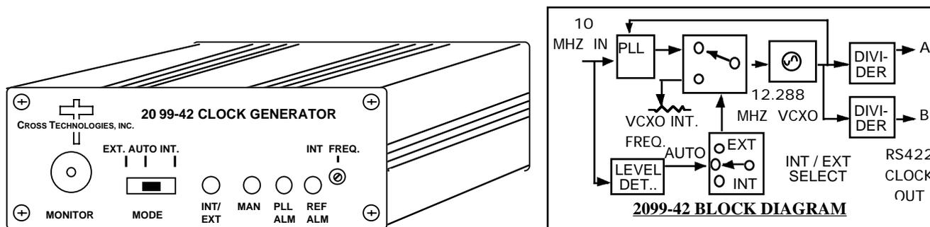
**FIGURE 1.1 2099-42 Clock Generator Block Diagram and Front Panel**
