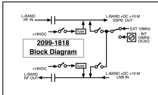
**FIGURE 1.2 Model 2099-1818 10MHz Source/Inserter Block Diagram**
