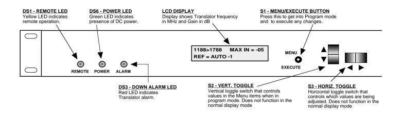
FIGURE 2.3 2083-0914 Front Panel Controls and Indicators
