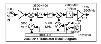
FIGURE 1.2 Model 2083-0914 Translator Block Diagram
