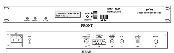
FIGURE 1.1 Model 2083-0914 Front and Rear Panels (Shown with optional Ethernet & Option E)
