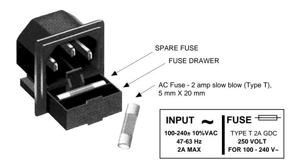
FIGURE 2.4 Fuse Location and Spare Fuse
