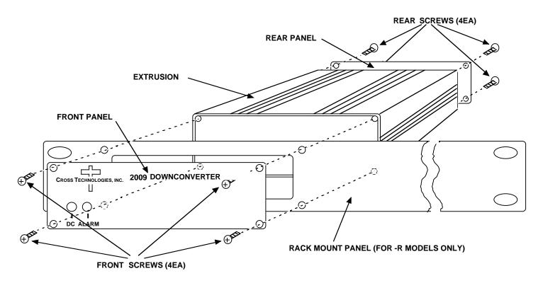
FIGURE 2.1 Model 2009-72P-79P Assembly (-R option shown)
