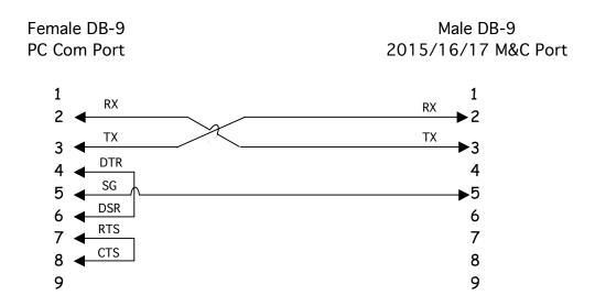
It's a little more complicated than a 'basic Crossover' (2-3, 3-2 (TX-RX)) with Signal Ground (pins 5-5) cable. On the PC Terminal side PINS 4 & 6 (DTR-DSR) need to be jumpered together and PINS 7 & 8 (RTS-CTS) also need to be jumpered together.
