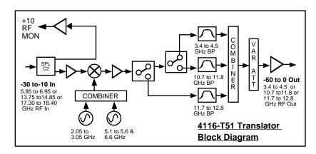
FIGURE 1. Model 4116-T51 Multi-Band Block Translator Block Diagram
