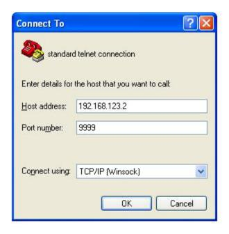
Figure 2-E: Telnet Settings in Hyper Terminal
