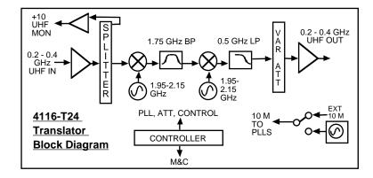
FIGURE 1 Model 4116-T24 Multi-Band Block Translator Block Diagram
