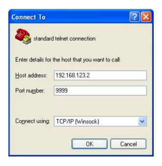
Figure 2-E: Telnet® Settings in Hyper Terminal
