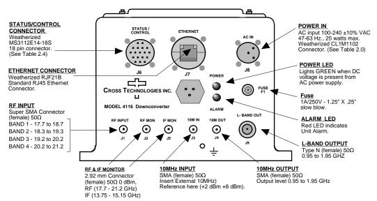
Model 4116-41-213 Ka-Band Block Downconverter Front Panel
