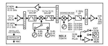
FIGURE 1.0 Model 4116-41-213 Ka-Band Downconverter Block Diagram
