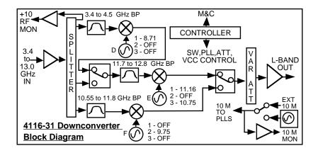
FIGURE 1. Model 4116-31 Tri-Band Block Downconverter Block Diagram
