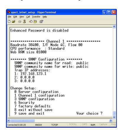
Figure 2-F: Device Server Configuration Menu
