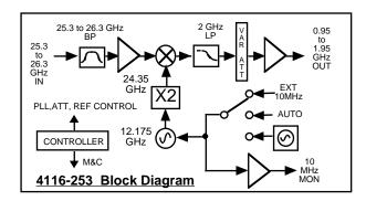
FIGURE 1. Model 4116-253 Ka-Band Block Downconverter Block Diagram
