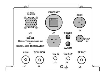
FIGURE 1. Model 4116-24T11, Translator Front Panel
