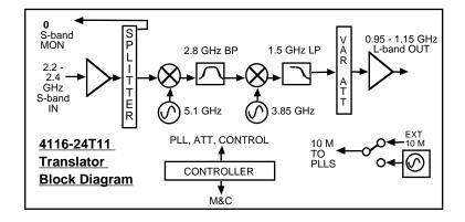
FIGURE 1A. Model 4116-24T11 Translator, Block Diagram
