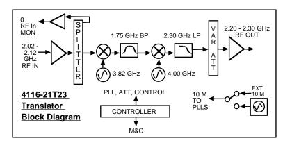
FIGURE 1A. Model 4116-21T23, Translator, Block Diagram
