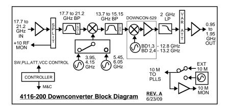
FIGURE 1 Model 4116-200 Ka-Band Block Downconverter Block Diagram
