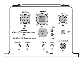
Model 4116-200 Ka-Band Block Downconverter Front Panel
