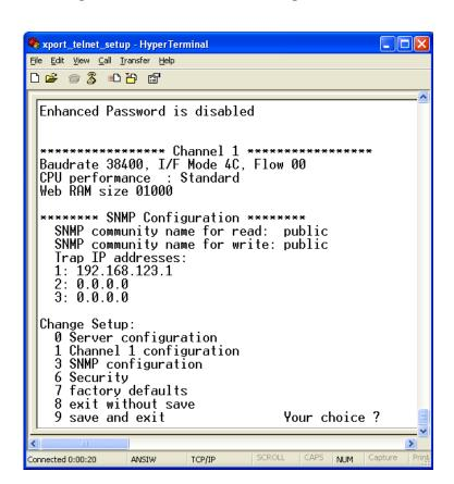
Figure 2-F: Device Server Configuration Menu
