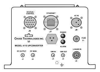
Model 4115-41-212 Ka-Band Block Upconverter Front Panel
