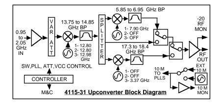
FIGURE 1.0 Model 4115-31 Tri-Band Block Upconverter Block Diagram
