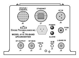
Model 4115-31 Tri-Band Block Upconverter Front Panel
