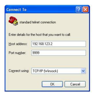
Figure 2-E: Telnet® Settings in Hyper Terminal
