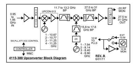
FIGURE 1.0 Model 4115-300 Ka-Band Block Upconverter Block Diagram
