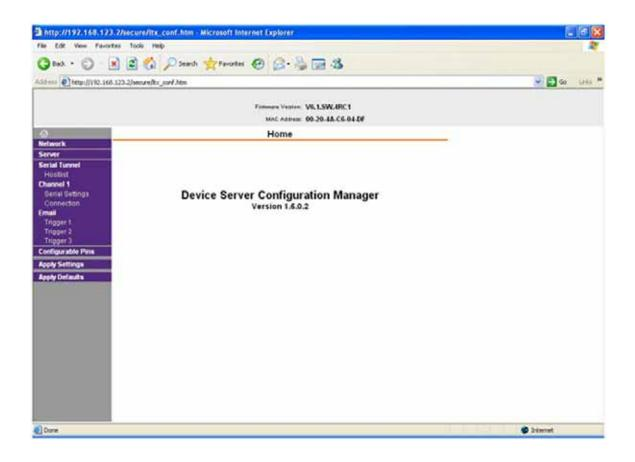
In the left frame of the configuration manager click on Network to display the Network Settings screen. Enter the IP address, Subnet mask, and Gateway address with delimiter dots (example: 192.168.192.47). Click on apply settings to apply the new settings in the device server.
