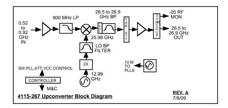
FIGURE 1B Model 4115-267 Ka-Band Block Upconverter, Block Diagram
