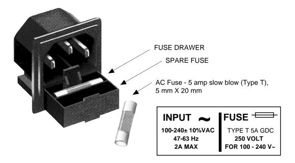
FIGURE 2.4 Fuse Location and Spare Fuse
