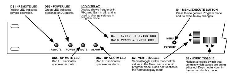
FIGURE 2.3 3116-T71 Front Panel Controls and Indicators
