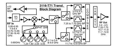
FIGURE 1 A Model 3116-T71 Multi-Band, Translator Block Diagram
