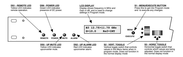
FIGURE 2.3 3116-T71-184 Front Panel Controls and Indicators
