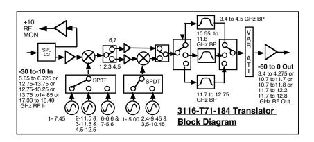
FIGURE 1.A Model 3116-T71-184 Multi-Band Translator Block Diagram
