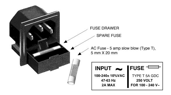
FIGURE 2.4 Fuse Location and Spare Fuse
