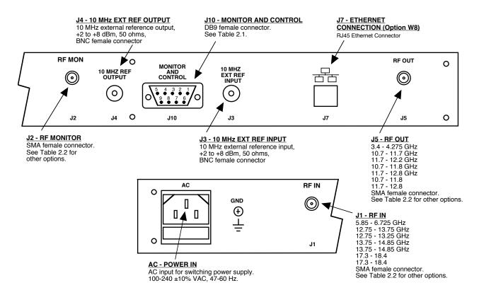
FIGURE 2.2 3116-T71-184 Rear Panel Inputs and Outputs
