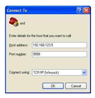
Figure 2-D: Telnet Settings in Hyper Terminal
