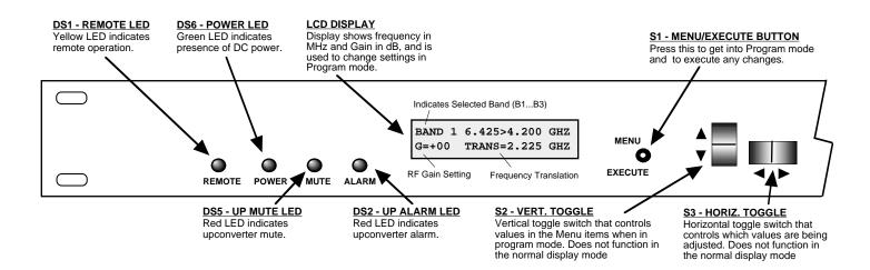
FIGURE 2.3 3116-T31-148 Front Panel Controls and Indicators
