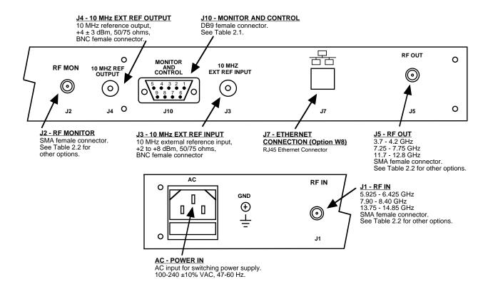
FIGURE 2.2 3116-T31-148 Rear Panel Inputs and Outputs
