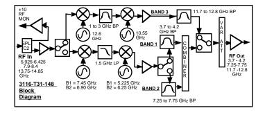
FIGURE 1-A Model 3116-T31-148 Block Diagram
