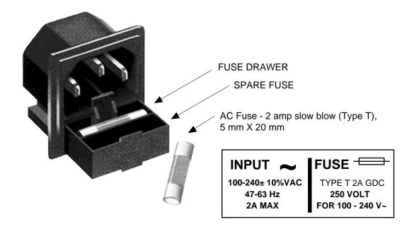
FIGURE 2.4 Fuse Location and Spare Fuse
