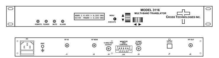
Figure 1. Model 3116-T31-148 Multi-Band Block Translator, Front & Rear Panels
