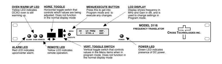
FIGURE 2.3 3116-T291 Front Panel Controls and Indicators
