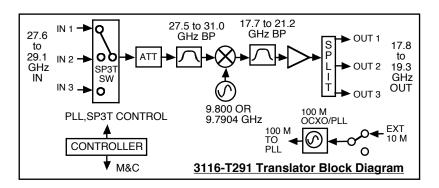
FIGURE 1A Model 3116-T291 Block Translator Block Diagram
