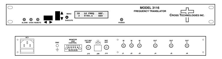
Figure 1.0 Model 3116-T291 Block Translator, Front & Rear Panels
