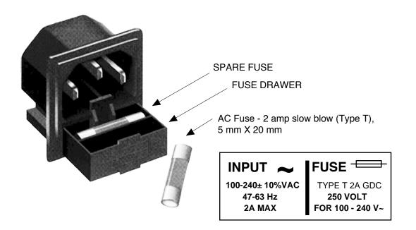
FIGURE 2.4 Fuse Location and Spare Fuse
