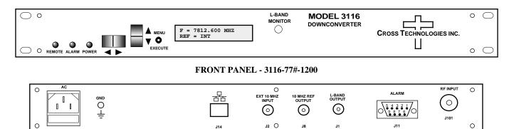
REAR PANEL - 3116-77#-1200 (Shown with optional RJ45 Ethernet Connector/J14)
