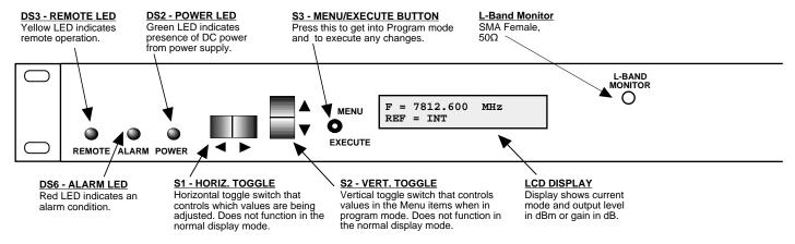
FIGURE 2.2 3116-77#-1200 Front Panel Controls and Indicators
