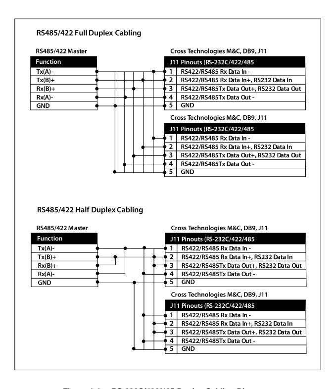
Figure 1.4 RS-232C/422/485 Duplex Cabling Diagrams
