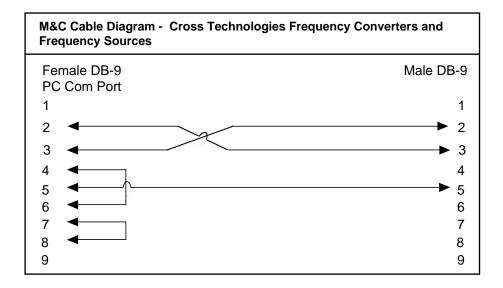
Figure 1.3 M&C Cable Diagram
