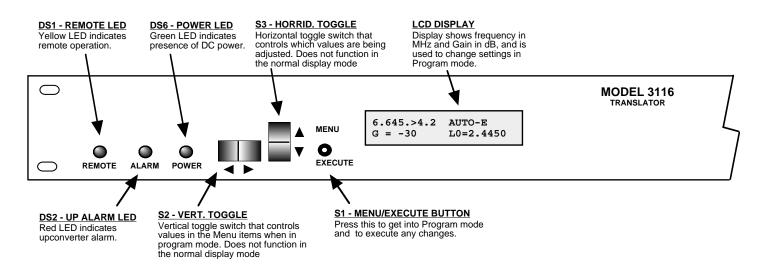
FIGURE 2.3 3116-66T42 Front Panel Controls and Indicators
