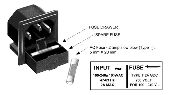
FIGURE 2.4 Fuse Location and Spare Fuse
