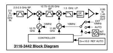
FIGURE 1.2 3116-3442 Block Diagram
