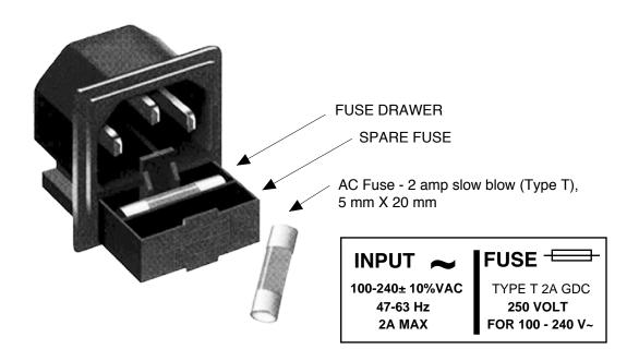
FIGURE 2.3 Fuse Location and Spare Fuse
