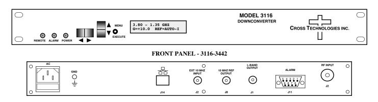
REAR PANEL - 3116-3442 (Shown with Optional RJ45 Ethernet Connector)
