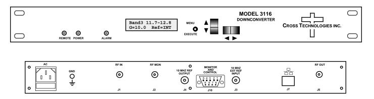
Figure 1. Model 3116-31 Multi-Band Block Downconverter, Front & Rear Panels
