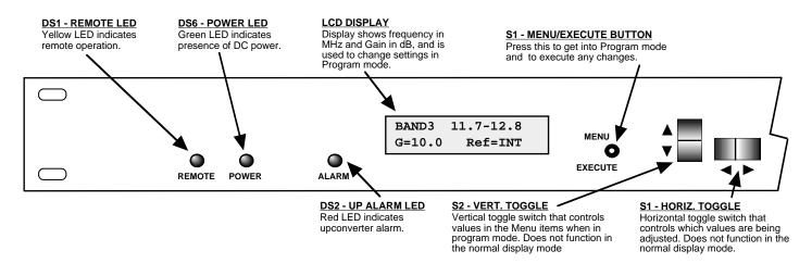
FIGURE 2.3 3116-31 Front Panel Controls and Indicators
