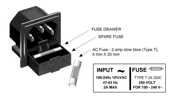
FIGURE 2.3 Fuse Location and Spare Fuse
