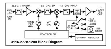
FIGURE 1.2 3116-277#-1200 Block Diagram
