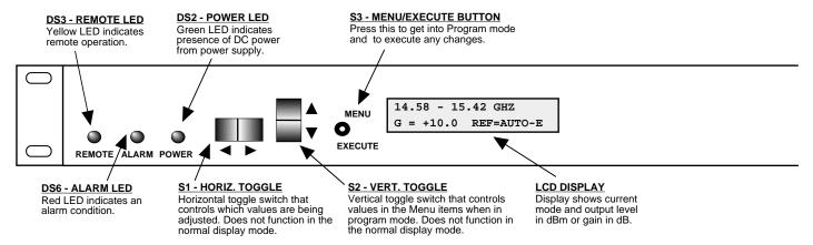
FIGURE 2.2 3116-145-1600 Front Panel Controls and Indicators
