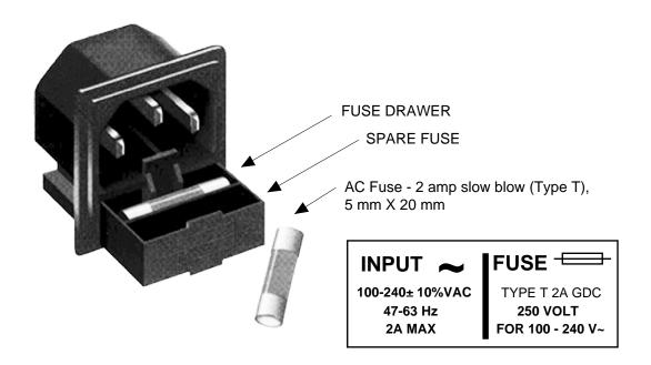
FIGURE 2.3 Fuse Location and Spare Fuse
