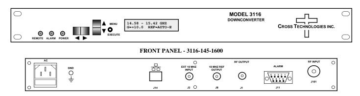
REAR PANEL - 3116-145-1600 (Shown with Optional RJ45 Ethernet Connector)
