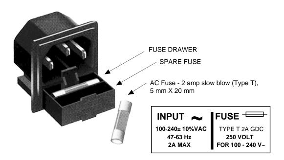
FIGURE 2.3 Fuse Location and Spare Fuse
