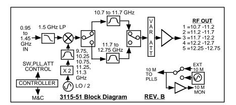
FIGURE 1 Model 3115-51 Block Upconverter Block Diagram
