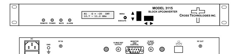
Model 3115-51 Block Upconverter Front Panel
