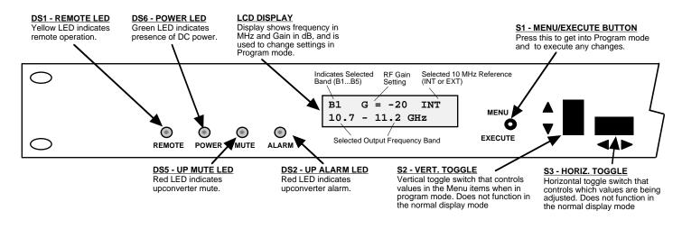
FIGURE 2.3 3115-51 Front Panel Controls and Indicators
