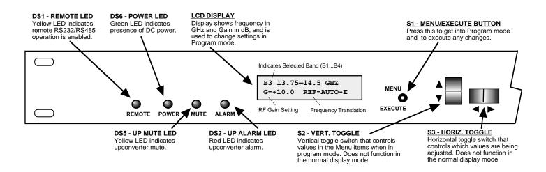
FIGURE 2.3 3115-41-184 Front Panel Controls and Indicators
