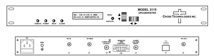
Figure 1. Model 3115-41-184 Multi-Band Block Upconverter, Front & Rear Panels
