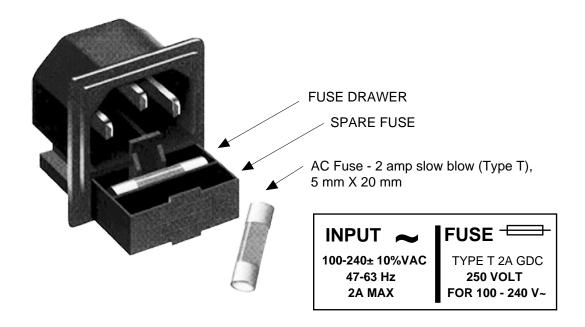
FIGURE 2.4 Fuse Location and Spare Fuse
