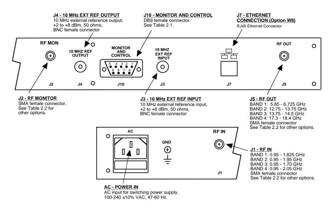
FIGURE 2.2 3115-41-184 Rear Panel Inputs and Outputs
