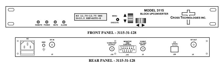
FIGURE 1.1 3115-31-128 Front and Rear Panels
