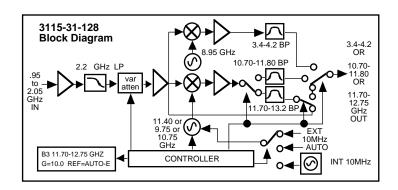
FIGURE 1.2 3115-31-128 Block Diagram
