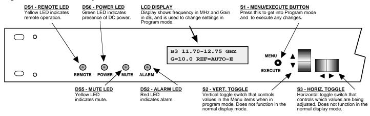
FIGURE 2.2 3115-31-128 Front Panel Controls and Indicators
