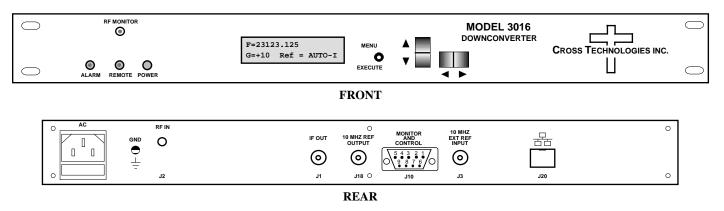
FIGURE 1.1 Model 3016-2124 Front and Rear Panels
