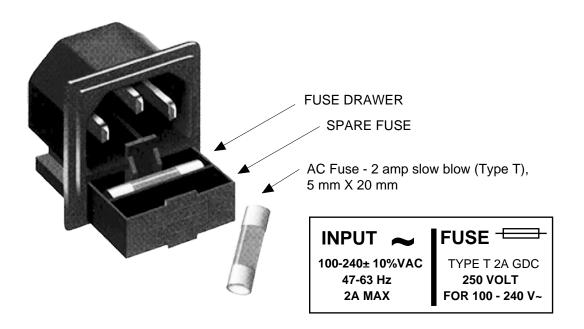
FIGURE 2.4 Fuse Location and Spare Fuse
