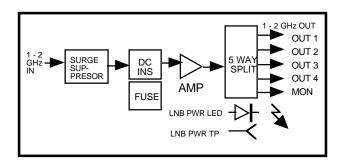
FIGURE 1.3 Model 284-15 RF Splitter Block Diagram
