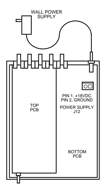
FIGURE 2.1 284-15 Mechanical Assembly
