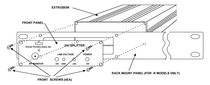
FIGURE 2.5 Rack Mounting The 284-15
