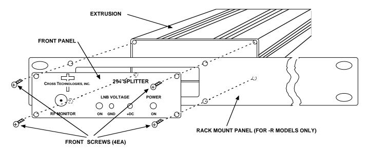
FIGURE 2.5 Rack Mounting the 284-09
