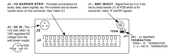
FIGURE 2.3 2710 Inputs and Outputs
