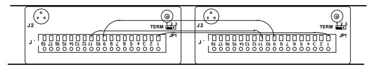
FIGURE 2.6 Model 27XX Rear Panels Showing DC wired together for Use With One Wall Power Supply
