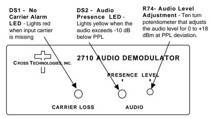
FIGURE 2.2 2710 Front Panel Controls and Indicators
