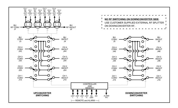
FIGURE 1.2 Model 2582-344 Switch Block Diagram
