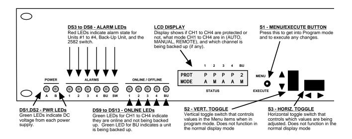
FIGURE 2.2 2582-344 Front Panel Controls and Indicators
