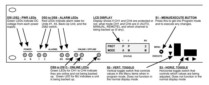
FIGURE 2.2 2582-324 Front Panel Controls and Indicators
