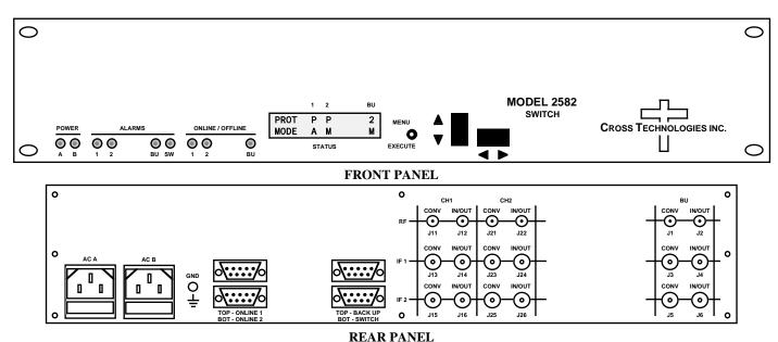
FIGURE 1.1 Model 2582-324 Front and Rear Panels
