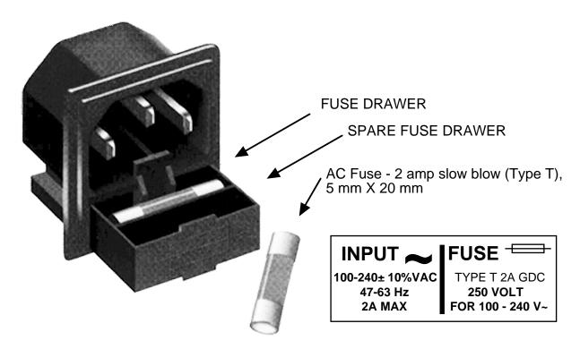
FIGURE 2.3 Fuse Location and Spare Fuse
