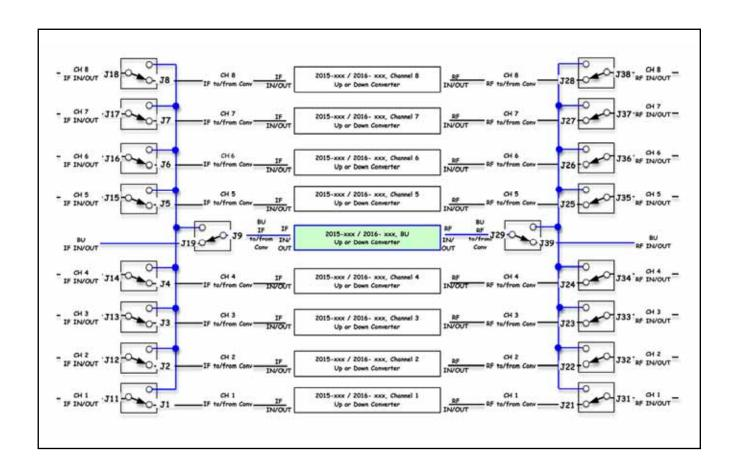
FIGURE 1.2 Model 2582-282 Switch Block Diagram
