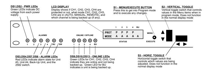
FIGURE 2.2 2582-142 Front Panel Controls and Indicators
