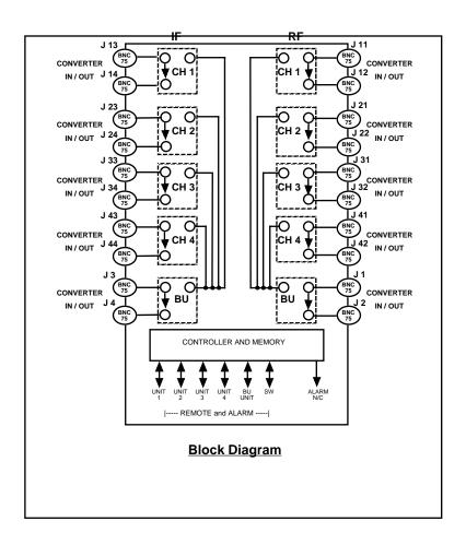
FIGURE 1.2 Model 2582-142 Switch Block Diagram
